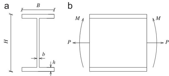
Fig. 2. (a): Section of beam, (b) an element subjected to external pull and bending moment.
