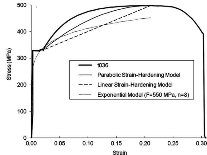
Fig. 1. Experimental stress-strain curve [19] and different models of mild steel.
