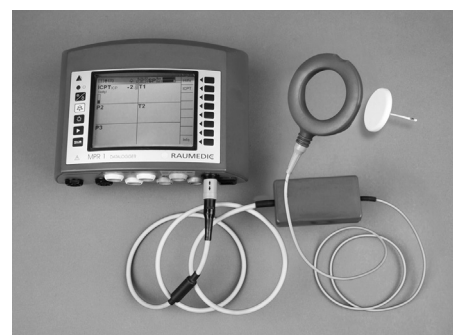
Figure 1. Hardware for telemetric measurement of intracranial pressure. The display and storage unit (Datalogger MPR-1) is connected to the antenna (Reader TDT1 readP). A cable-free connection for transmission of intracranial pressure data can be established by placing the reader unit close to the implant (Neurovent P-tel).
