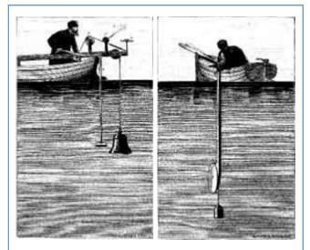
Figure 1. Jean Daniel Colladon uses an underwater church bell as a transducer to calculate the speed of sound through water.
