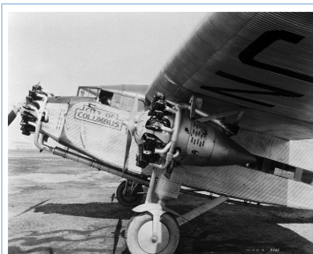
Figure 2. Ford Tri Motor equipped with 3 Pratt & Whitney Wasp engines with 420 horsepower each. Weight was 13,500 pounds, capacity was 13 to 15 passengers. This was the first real passenger plane in the U. S. (Reprinted with permission from the National Aeronautics and Space Administration.)
