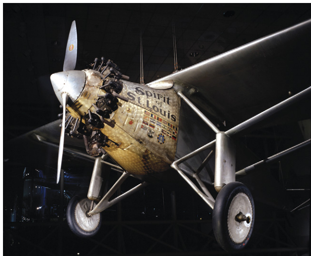
Figure 1. Charles Lindbergh fitted his Ryan NYP, Spirit of St. Louis , with a reliable air-cooled Wright J-5C engine, a type designed originally for the U.S. Navy. (Reprinted with permission from the National Air and Space Museum.)
