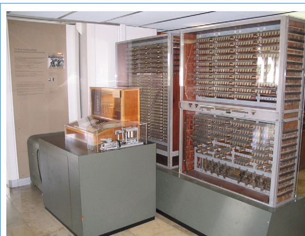
Figure 1. The Zuse Z3 is considered the world's first operational computer. Built by Konrad Zuse in 1941, it was programmable, was fully automated, and was later shown to be Turing complete. Program code and data were stored on punched film. (Original by Venusianer. Republished under the GNU Free Documentation License without alterations or additions.)
