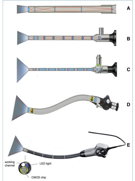
Figure 1. Types of endoscopes. (A) Initial lens scope with external illumination (Nitze & Bénèche, 1877). (B) Traditional lens scope. (C) Hopkins rod lens endoscope. (D) SELFOC lens (Nippon Sheet Glass, Tokyo, Japan) rigid endoscope ("needle scope" based on gradient fiber). (E) Flexible fiberscope. (Endoscopes depicted in B–E are used with external cold light and fiberglass light cable.) (F) Video-endoscope ("chip-in-the-tip"), with integrated LED light.
