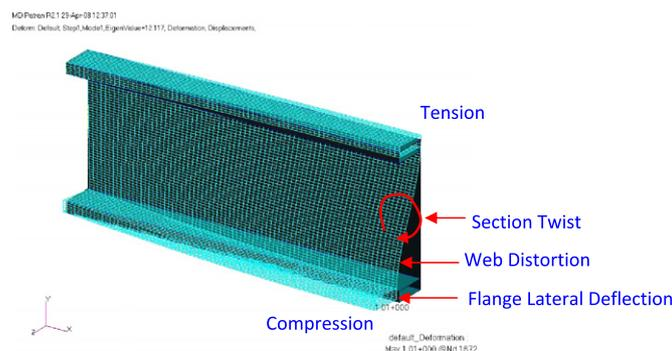
Fig. 3. Lateral distortional buckling of LSBs.
