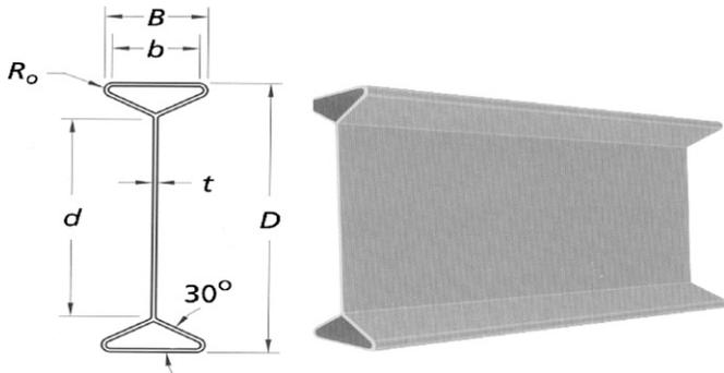
Fig. 1. Hollow flange beams.
