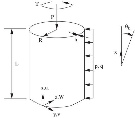
Fig. 1. Shell geometry, coordinate system and applied loading.
