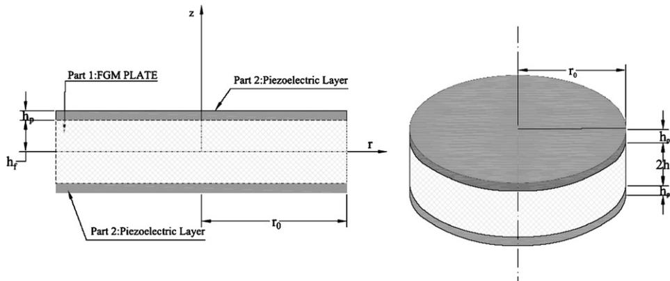
Fig. 1. Schematic representation of the FGM circular plate with two piezoelectric layers mounted on its upper and lower surfaces.
