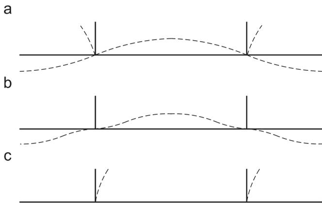
Fig. 2. Basic local buckling modes, (a) combined plate and stringer buckling, (b) limit case I: plate buckling in the case of stiff stringers, (c) limit case II: stringer buckling in the case of stiff plate.
