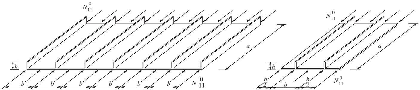
Fig. 1. Compressively loaded composite plate stiffened by blade stringers (left portion), representative unit cell for local buckling analysis (right portion).
