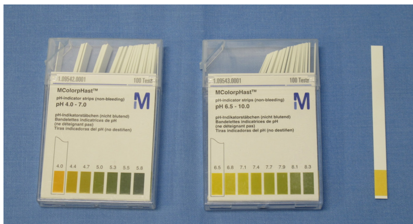
Fig. 1 – pH indicator strips. The pH indicator strips used in this study were MColorpHast™ (Merck KGaA, Darmstadt, Germany; pH 4.0–7.0 and 6.5–10.0).
