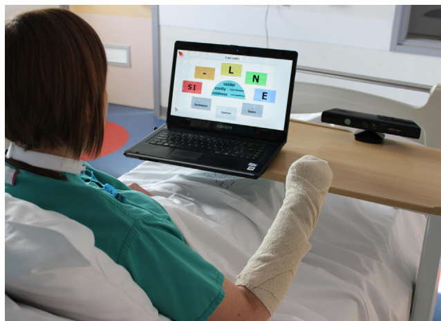
Fig. 2 – Use of the Kinect™ arm movement tracking system. Via the Kinect™ gaming sensor on right of the image the software on the attached laptop computer collects information on the outline of the right arm, tracking its movement to control an on-screen pointer to select letters and create words.
