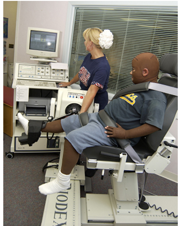
Fig. 1 – Image showing the Biodex Isokinetic Dynamometer. Subjects are seated upright with seat height, distance from ankle to knee and distance from knee to back recorded.
