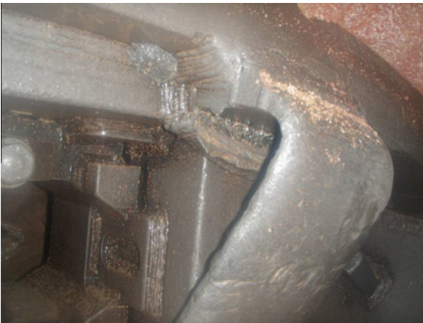
Fig. 2. Damaged (bent and abraded) mixing arm, slurry TBM.
