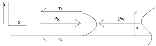
Fig. 1. Grout flow through a rock joint.
