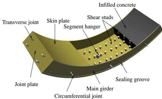
Fig. 1. Schematic of composite segment.
