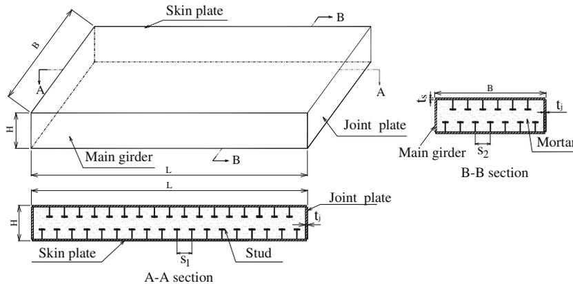
Fig. 2. Detail of composite segment specimen.
