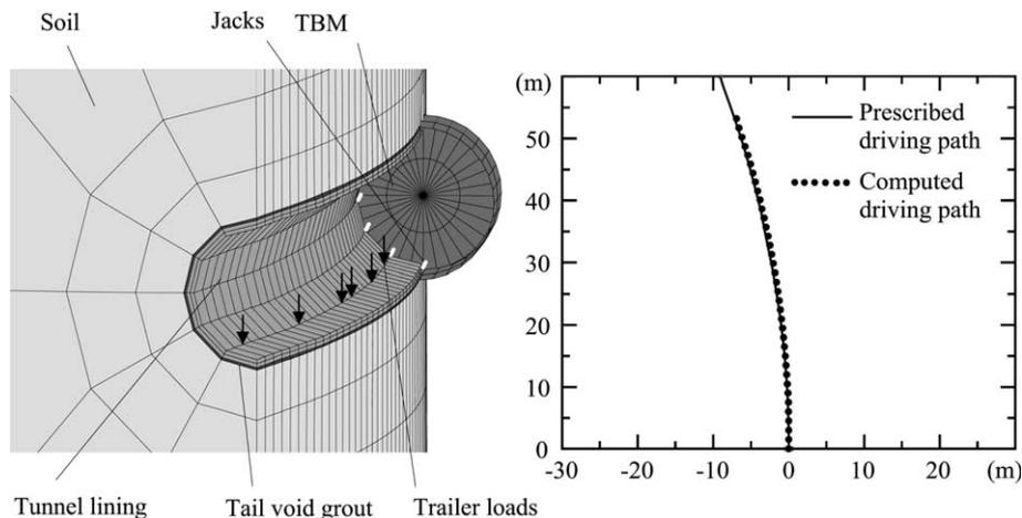
Fig. 1. Test simulation of a curved shield tunnel advance with a radius of 200 m.
