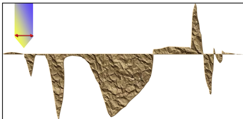
Fig 1. Various methodologies are used to assess roughness. This is a graph of the profilometry with a stylus method demonstrating the problems in assessing the actual variations of peaks and valleys on a surface, establishing the limiting factor of stylus size.
