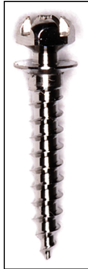
Fig 1. The self-drilling miniscrew used in this study: screw thread length, 8 mm; total length, 11 mm; internal diameter, 1.2 mm; external diameter, 1.6 mm.
