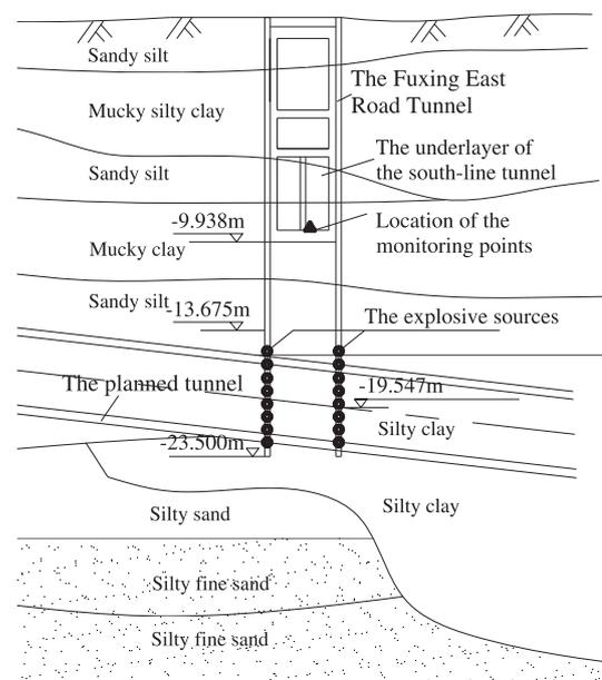
Fig. 2. Typical cross section of the Puxi terminal segment of the Fuxing East Road Tunnel.
