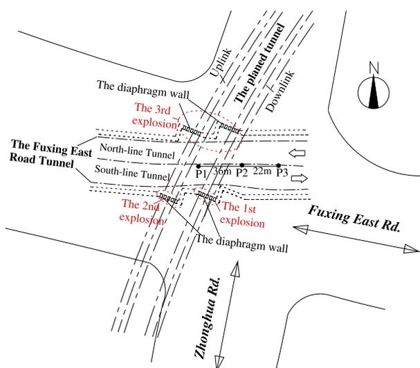
Fig. 1. Plane view of the Fuxing East Road Tunnel and the planned subway tunnel.
