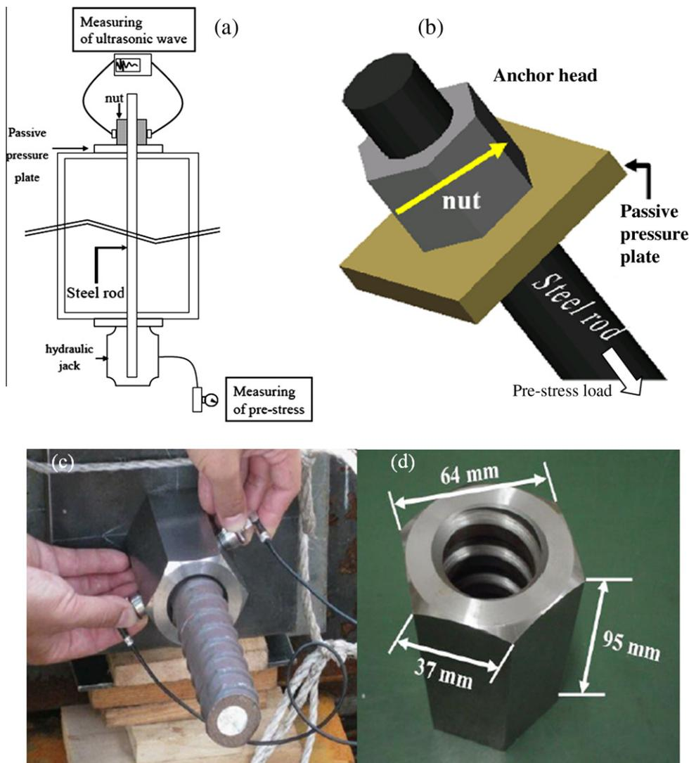
**Fig. 1.** (a) Schematic representation of pre-stress, (b) wave propagation through the nut, (c) photograph of the experiment and (d) details of the nut used in the anchor head.
