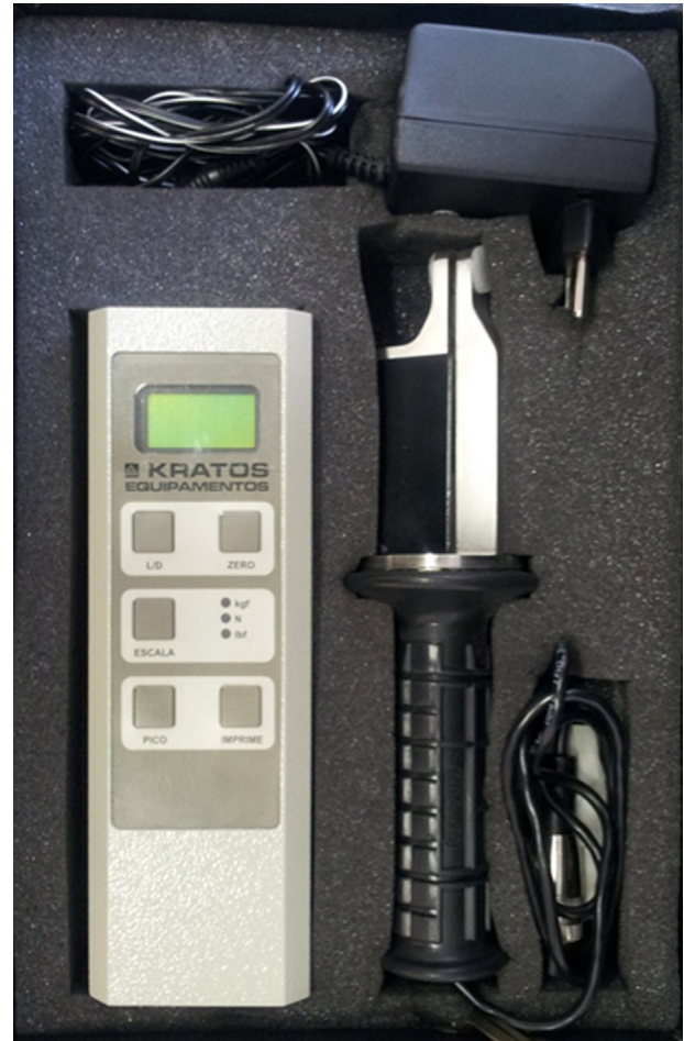
Fig. 1. Gnathodynamometer used to perform the measurements (digital dynamometer, IDDK model, Kratos, Bauru, SP, Brazil).
