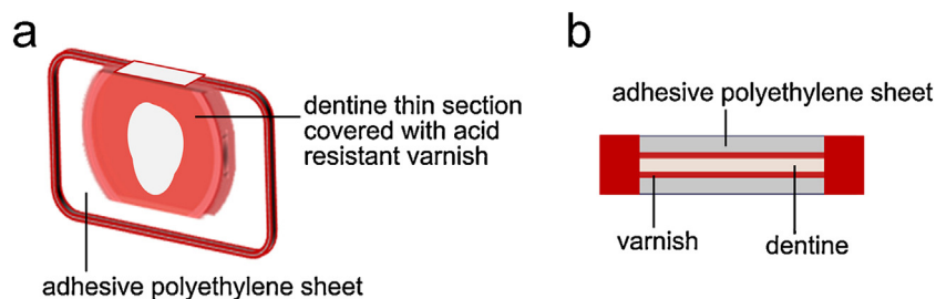
Fig. 1. Schematic representation of the modified dentine single thin-section technique used in this study. (a) Thin dentine section covered in acid-resistant varnish and adhesive polyethylene sheet. (b) Coronal view of the specimen showing the different coating layers used in the specimen preparation.
