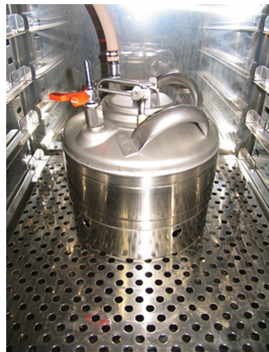
Fig. 2 – The pressure device in the incubator. PDL cells were continuously compressed by this device.
