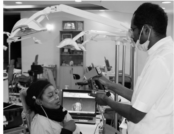
Fig. 1. The instrument (portable laser scanner) being used to image the face of a young woman. The digital representation of the woman's face can be seen on the computer screen.
