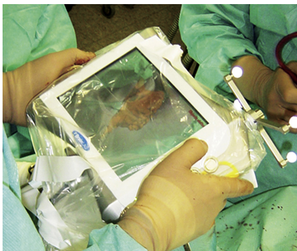
Fig. 1. Surgeon's view through the portable, interactive, image-guided, visualisation display. The maxilla was virtually augmented as a three-dimensional object in its new position.
