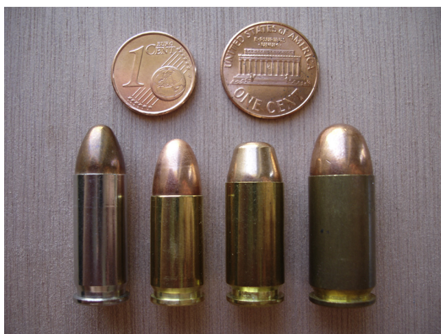
Fig. 1. Examples of pistol ammunition. From left to right: .38 Super; 9-mm Luger; .40 Smith & Wesson (S&W); .45 Automatic Colt Pistol (ACP). The former two are essentially of the same diameter, but the .38 Super is more powerful as indicated by its considerably longer cartridge case containing larger propellant charge. Note also the truncated ‘semiwadcutter’ (SWC) configuration of the .40 S&W compared to the more common round nose shape of the other bullets. (One cent coins are shown for comparison.)
