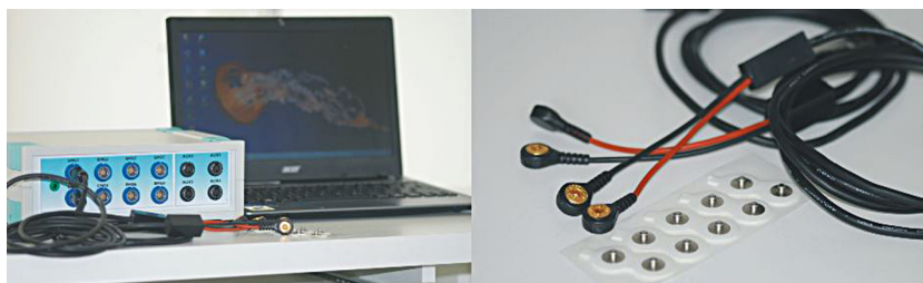
Fig. 1. MyosystemBr1 electromyograph and bipolar surface electrodes.
