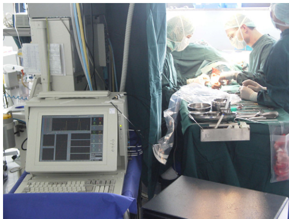
Fig. 1. O2C in the operating room, well integrated while a flap is being raised, presenting microvascular parameters online.
