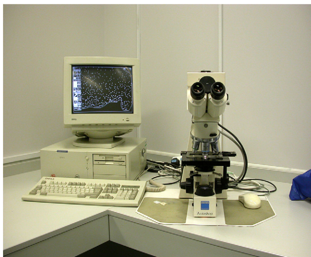
Fig. 1. AxioHome interactive microscope system, showing computer screen analysis of cyclin A-labelled dysplastic epithelium.
