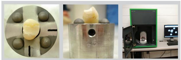
Figure 1. A premolar is secured in a stainless steel ring (left and middle) and scanned with an optical scanner (Comet xS, Steinbichler Optotechnik, Neubeuern, Germany) (right).
