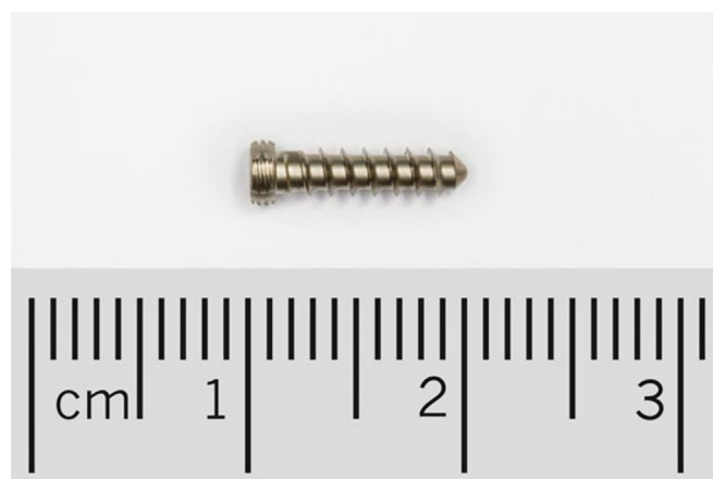
Fig. 3. 2.0 Synthes: 10 mm self-taping and self-drilling screws with conical double threads beneath the screw head.
