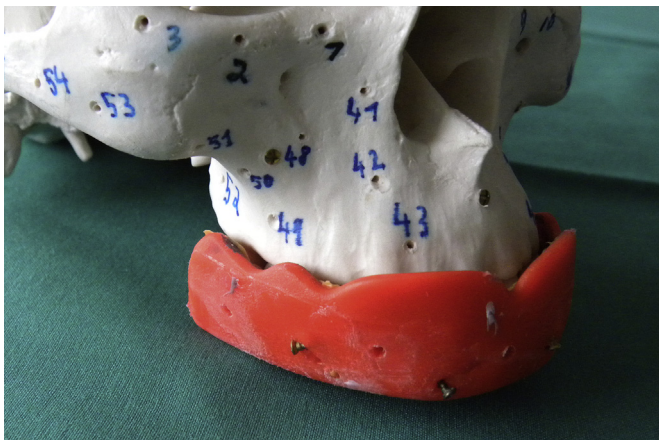
Fig. 1. Skull model with mounted rapid splint.
