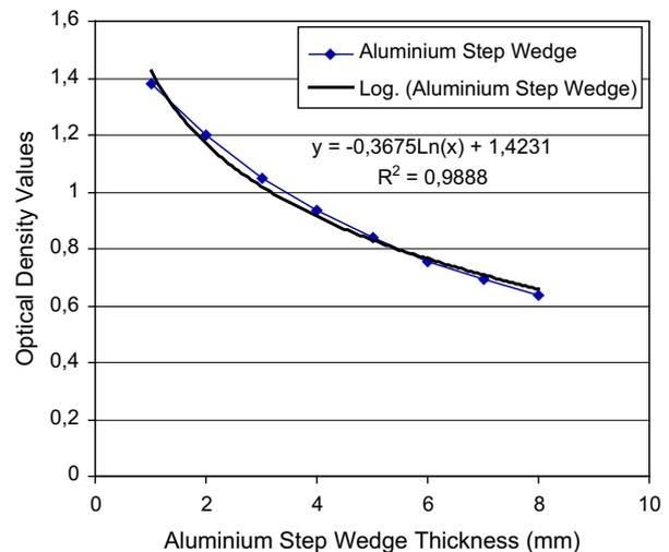
**Fig. 1.** Optical density calibration curves for Al step wedge.
