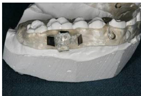
Fig. 1 – The orthodontic appliance with a custom made retainer for the Ge crystals.
