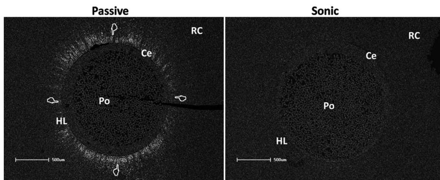
**Figure 1.** Representative scanning electron microscopic images of the post–cement–adhesive root interfaces bonded of XP Bond+self-activator/Enforce in the cervical third. The white hands indicate the regions where silver nitrate uptake was measured. When the adhesive was applied manually (passive), the amount of silver nitrate uptake was higher and occurred at all bonded interfaces. This was minimal with sonic application. Ce, resin cement; HL, hybrid layer; Po, fiber post; RC, root canal.
