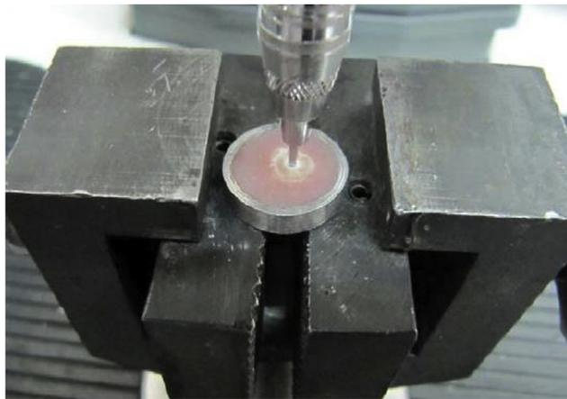
**Figure 1.** The experimental design and application of push-out force.
