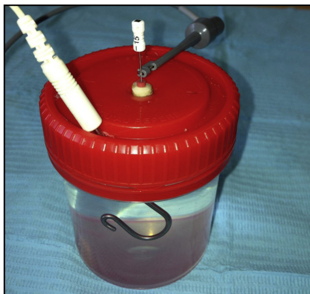
Figure 1. A screw top plastic container was filled with 0.9% NaCl solution; the tooth and the lip clip of the EAL were inserted through the screw top by 2 self-made holes.
