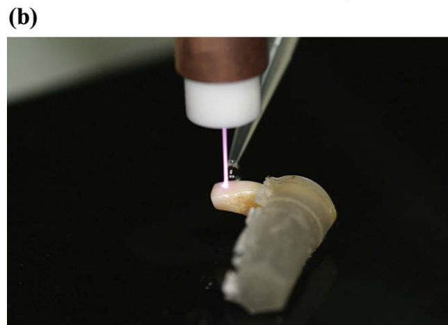
Figure 1. Configuration (a) of the tooth bleaching experiment and schematic of the plasma device and (b) of the process.
