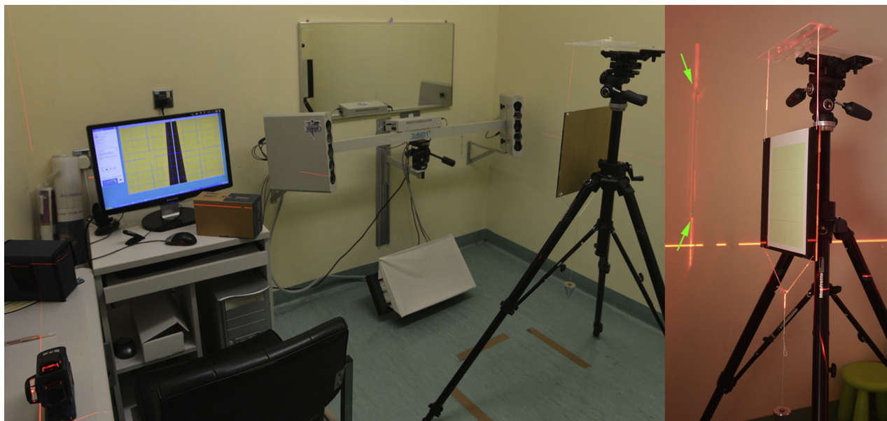
FIGURE 1. Left , The hanging reference board is placed at the capturing position, which is aligned parallel to the mirror using the alignment laser. The graph paper on the board indicates the roll angles needed to rotate the digital models back to true vertical. Right , When the board is aligned to face the mirror, the laser beam creates shadows (green arrows) on the right wall from the threads at which they overlap. The size of the board shadow is minimal.
