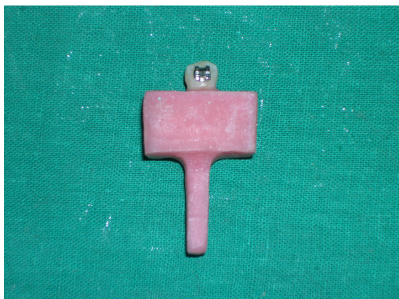
Fig. 1 – Sample being tested. Tooth mounted in acrylic block and bonded.
