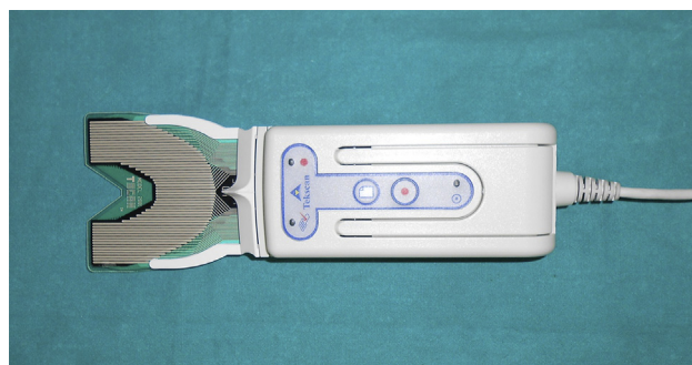
Fig. 1 – T-Scan III recording handle connects directly to a computer via a USB interface.
