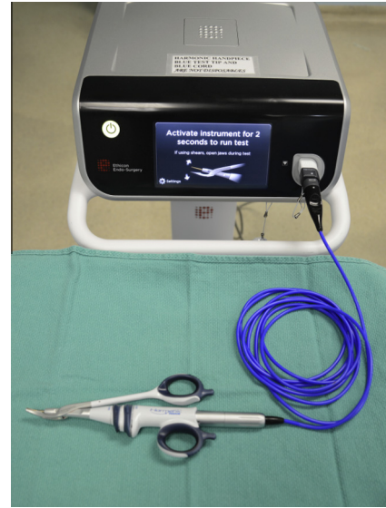
Figure 2 FOCUS Harmonic scalpel handpiece and console.
