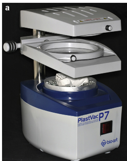
Fig. 2 – a. Model placed in the vacuum plasticizer; and b. Anterior view of the areas to be cut with disc.
