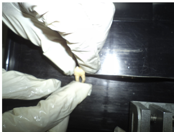
Fig. 1. The transversal section was made at cemento-enamel junction dividing the root and coronal portions with the help of Digital low speed cutting saw (MTI Corp; USA) under water spray.
