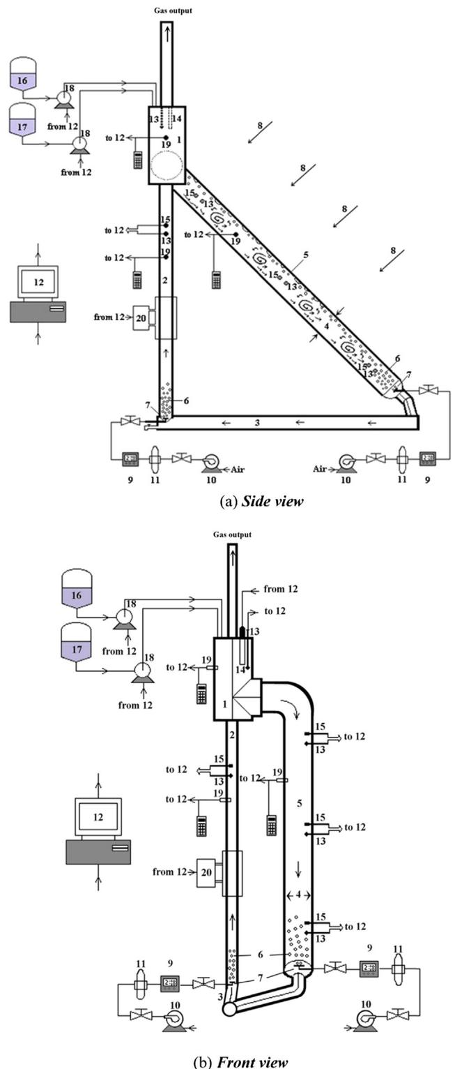
**Fig. 1.** Schematic of external airlift loop photobioreactor. 1: Separator; 2: Vertical side, riser; 3: Horizontal side; 4: Diameter of hypotenuse; 5: Hypotenuse, downcomer; 6: Bubble; 7: Bubble sparger; 8: Light source; 9: Digital gas flow meter; 10: Compressor; 11: Gas sterilizer, filter; 12: PC; 13: Thermometer; 14: Heater; 15: pH probe and controller; 16: NaOH solution; 17: HCl solution; 18: Dosing pump; 19: Dissolved oxygen (DO) sensor; 20: Heat exchanger.
