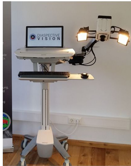
Fig. 1. Hyperspectral camera mounted at a flexible medical cart system.
