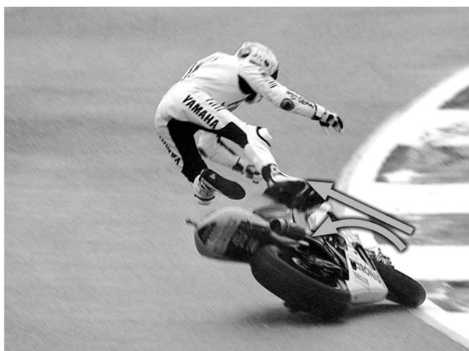
Fig. 2. Highside crash. Arrows represent force vectors. Copyright DORNA 2015. Reprinted with kind permission.
