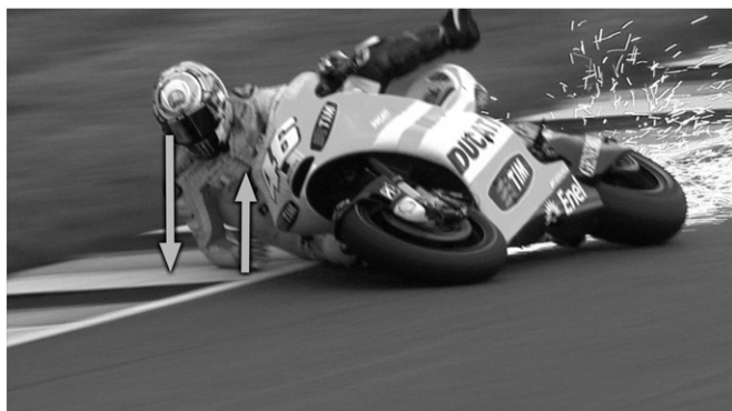
Fig. 1. Lowside crash. Arrows represent strength and direction of force vectors. Copyright DORNA 2015. Reprinted with kind permission.
