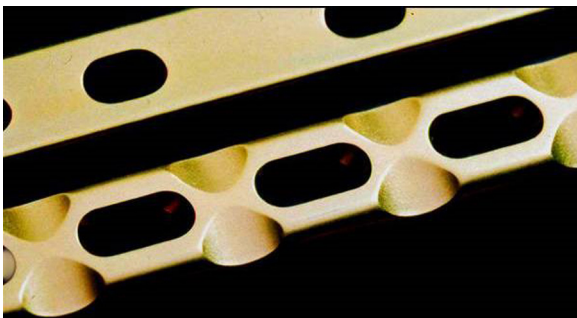
Fig. 1. Dynamic compression plate (DCP; top) and limited contact dynamic compression plate (LC-DCP; bottom). In the LC-DCP design the area of plate-bone contact (footprint) is greatly reduced thus improving cortical perfusion. Images reproduced with kind permission of the Copyright by AO Foundation, Switzerland [12].
