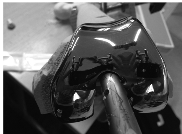
Fig. 1. Example of the scratches sustained to the retrograde femoral intramedullary nail on insertion through the femoral TKR component.
